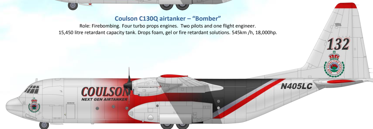
Lockheed L100-30 (382G) airtanker – "Bomber" Role: Firebombing. Four turbo props engines. Two pilots and one flight engineer. 15,450 litre retardant capacity tank. Drops foam, gel or fire retardant solutions. 545km/h, 18,000hp.
