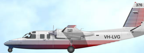
Rockwell Turbo Commander 690B – "Birddog" Role: Supervision & Reconnaissance. Two turbo prop engines. Single pilot. Agency Air attack supervisor, Radios and Satellite communications. 500km/h, 1430hp.
