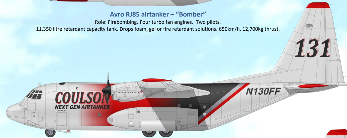
Coulson C130Q airtanker – "Bomber" Role: Firebombing. Four turbo props engines. Two pilots and one flight engineer. 15,450 litre retardant capacity tank. Drops foam, gel or fire retardant solutions. 545km/h, 18,000hp.
