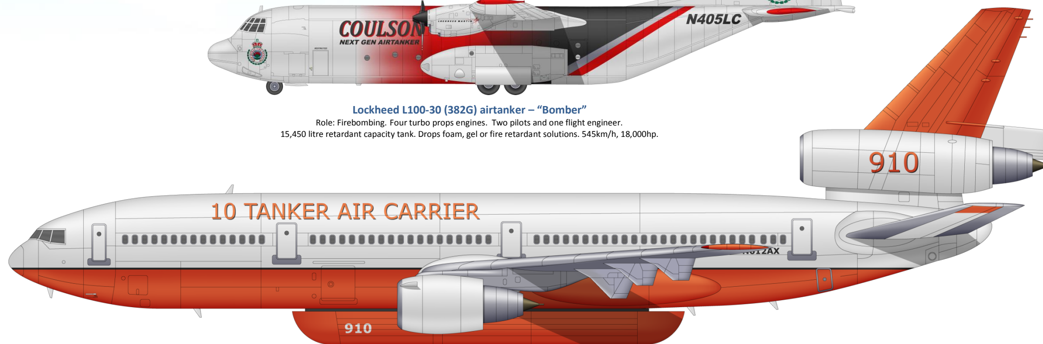
McDonnell Douglas DC-10-30 airtanker – "Bomber" Role: Firebombing. Three turbo fan engines. Two pilots and one flight engineer. 43,900 litre retardant capacity tank. Drops foam or fire retardant solutions. 650km/h, 70,000kg thrust.
